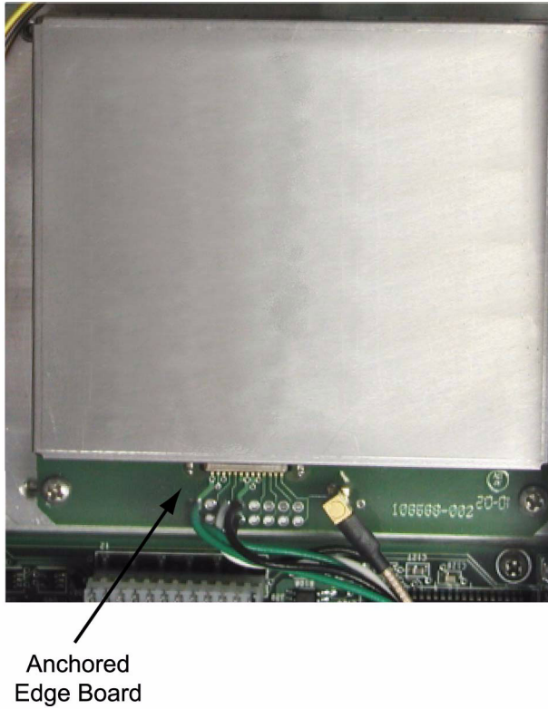
Figure 2-6 Anchored Edge Board Mounting Example
